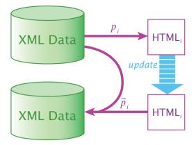
Figure 2. Bidirectional transformation between XML data and HTML sources
