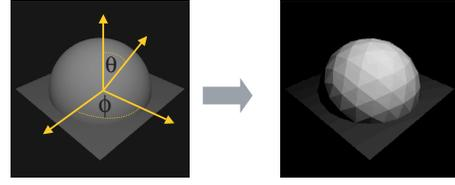
illumination distribution of a scene is approximated by discrete sampling over the entire surface of the extended light source.
