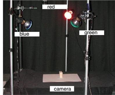
Figure 8: Experimental setup with three area light sources with different colors
