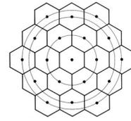
Figure 6: Hexagonal grids used for supersampling inside one light source
