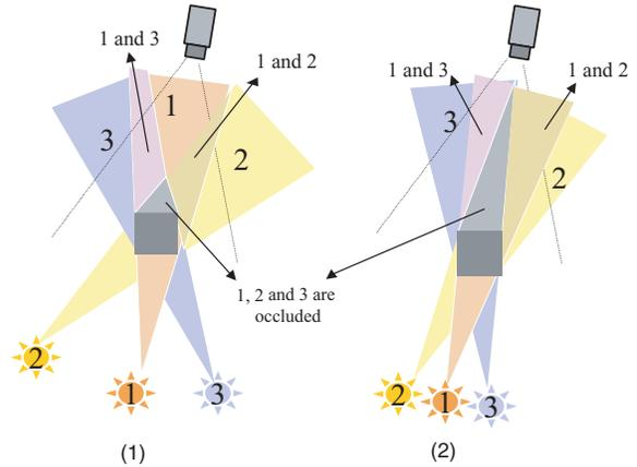
Figure 4: Difference in visible combinations of occlusions of lights: (1) coarsely distributed light sources and (2) densely distributed light sources
