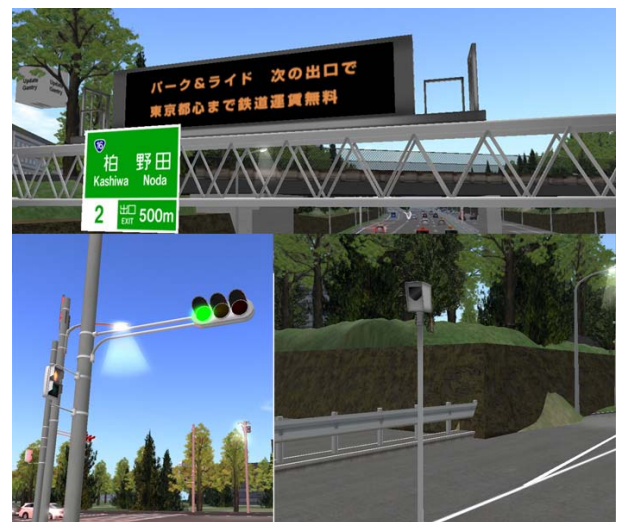
Figure 3: Virtual representations of objects manipulated by X-Roads: a gantry for customized message display (top), a traffic light (bottom-left), and a sensor (bottom-right).
