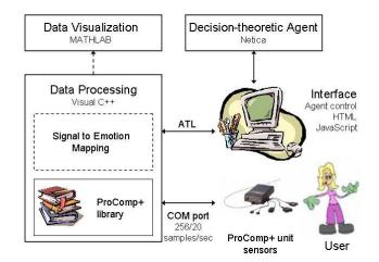
Fig. 3. System architecture.
