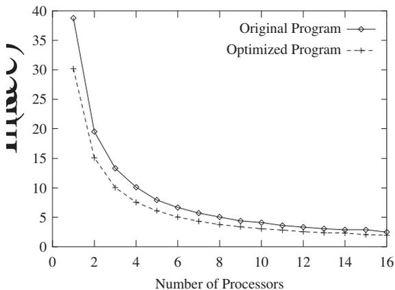
Fig. 6. The computation time before/after the optimization.
